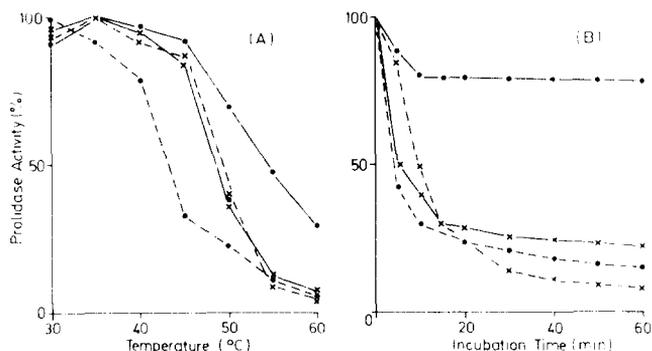
Fig. 4. Heat stability of control (—) and Case 2 (---) prolidase activity against phe-pro without (○) or with (●) 1.33 mmol/l  $Mn^{2+}$ . A. Effect of 5 min at 30–60°C. B. Effect of preincubation at 48°C for up to 60 min.
